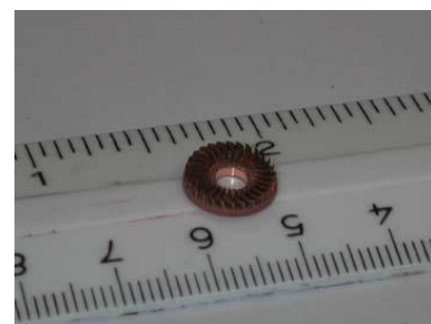
Figura 10. Microturbina in rame.
