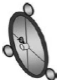
Hoop supported sail with hoop control vanes and payload suspended on a web.
